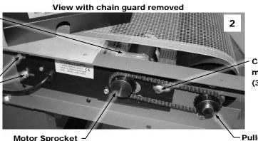
Control assembly mounting screw (3 total)
